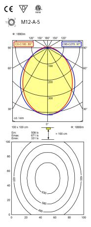
light source LED work equipment without connected load 22-26 V, DC env. 15 W power consumption luminous flux approx. 1.890 lm luminous efficiency approx. 126 lm/W light type/-color cold white colour temperatur approx. 5.000 K CRI > 80 color rendering index light distribution direct beam angle 89° / 97° chromaticity tolerance LED < 4 SDCM glare control screen system of protection IP 54 class of protection
